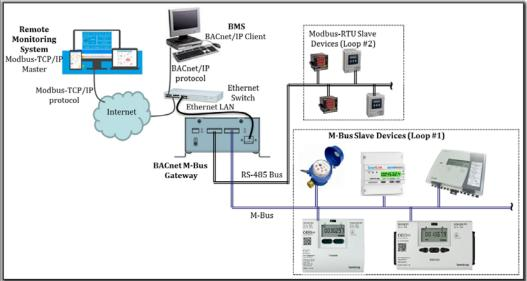
A typical application scenario with M-Bus BTU Meters on a multi-drop network and Modbus-RTU(connected on RS-485 multi-drop network) field devices connected through the Gateway to a BACnet based BMS and in parallel with a Modbus based remote monitoring system is shown in the picture. The BACnet/IP Device Server in the Gateway makes all the data-points accessed from all the configured M-Bus and Modbus-
