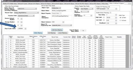
BACnet device. This BACnet/IP device server, running in the Gateway, is then accessed by any BACnet/IP BMS Client software and use it to indirectly read data-points in the M-Bus devices and read/write to the data-points in the Modbus devices.
